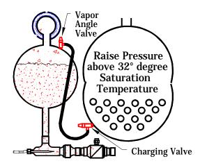
Figure 10. - Breaking Vacuum in chiller
