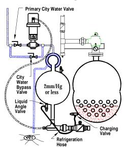
Figure 7. - Liquid Refrigerant being transferred to Containment Vessel
