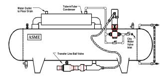
Figure 5. - Water Connections
