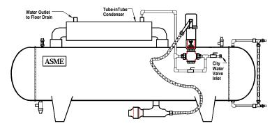
Figure 5. - Water Connections
