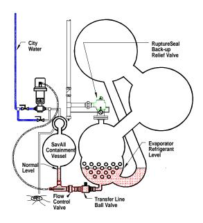
Figure 1. - Chiller Idle, Pressure Normal
