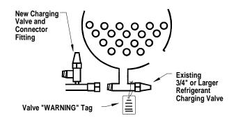
Figure 6. - Using New Charging Valve
